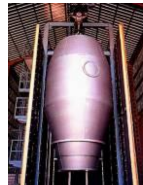
Superficial shotblasting process for the drum carried out in cubicles.
