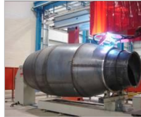
Incorporation of the latest developments in automatic welding and cutting processes.
