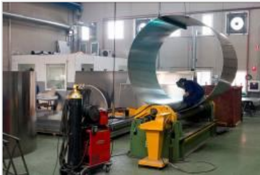
Shell manufacturing by means of a three-roller bending machine.
